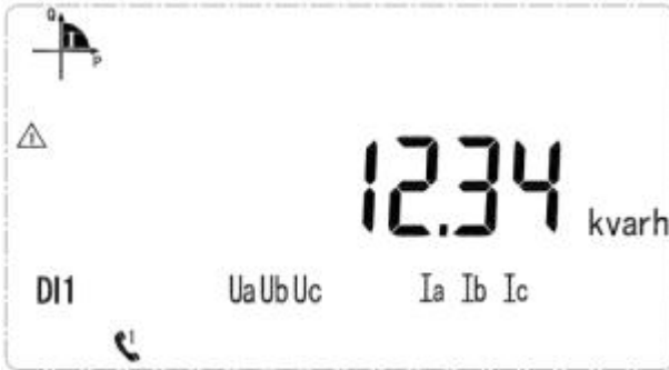
Current forward reactive energy 12.34kWh
